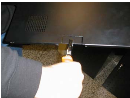
Cut the rear wall to make a hole for Damian Piccola to connect the communication cable. Install again the rear wall of the XS H - XS H/LIONESS vending machine.
